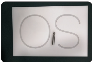
用匹配的铣槽刀在安装板上开好槽
