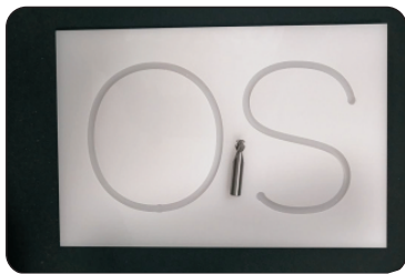
用匹配的铣槽刀在安装板上开好槽
